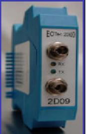
The 2D09 Optical Interface Module connects the EOTec 2000 modem with the fiber cable network allowing the optical signals to be transmitted to and received from another fiber optic modem. The 2D09 has the added benefit of supplying a 4 to 20mA output that is proportional to the optical power received from the remote location. This output can be used to diagnose fiber degradations before they become a "loss of signal" problem.
